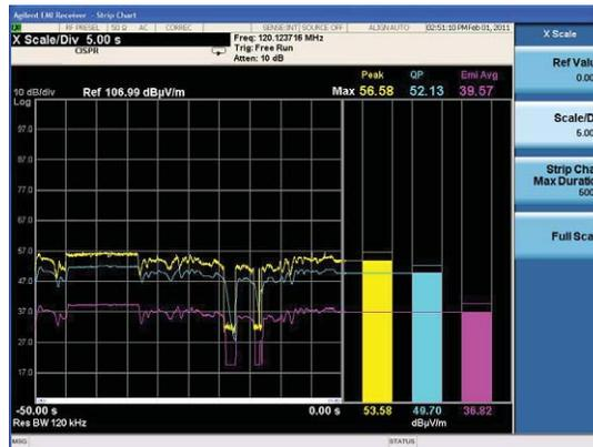
Strip Chart view provides a unique, gapless view of simultaneous detector response and is useful for tracking DUT performance as a function of turntable or antenna position
