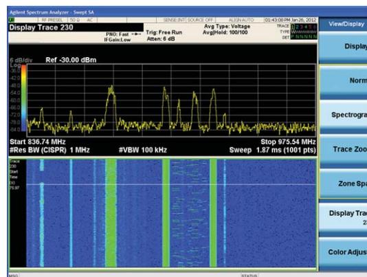
Spectrogram analysis allows users to understand both the amplitude- and time-varying nature of emissions using signal marker capability
