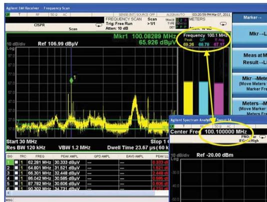
Use Global Center Frequency to move seamlessly between receiver and signal analyzer
