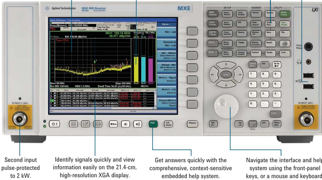
Second input pulse-protected to 2 kW. Identify signals quickly and view information easily on the 21.4-cm, high-resolution XGA display. Get answers quickly with the comprehensive, context-sensitive embedded help system. Navigate the interface and help system using the front-panel keys, or a mouse and keyboard.
