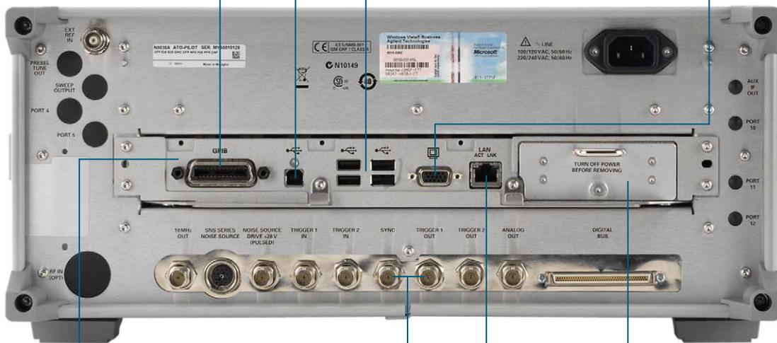
Removable CPU enables processor, memory, and I/O upgrades. Synchronize other test equipment with the analyzer using the external trigger output signals. Control the MXE remotely over 1000Base-T LAN. Removable solid-state drive. Additional solid-state drive available for instrument security.
